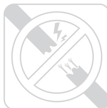
Check for damaged wires
